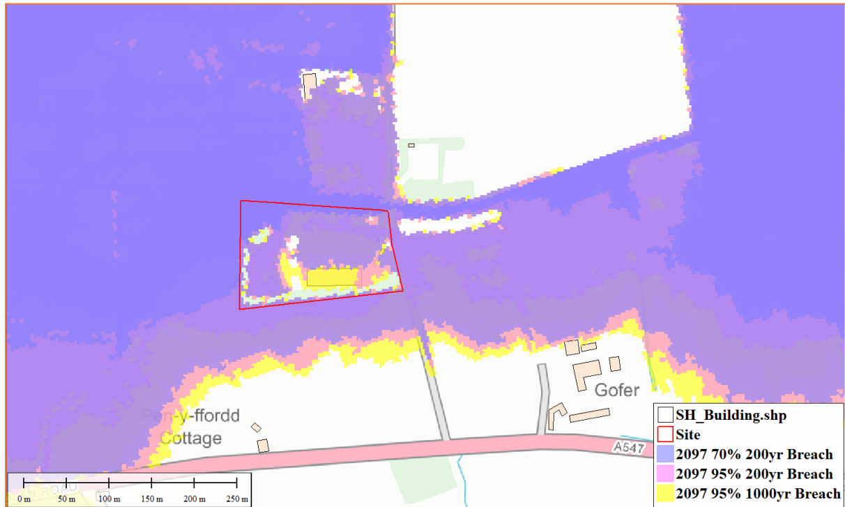
Figure 13: Modelled Maximum Breach Extents (Source: NRW, OS Mapping, Proposed Site plan)
