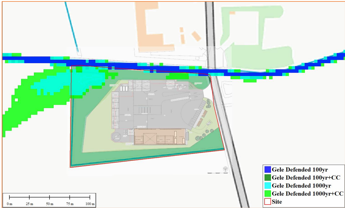
Figure 7: Modelled Afon Gele Defended flood extents at the site (Source: NRW, OS Mapping, Proposed Site plan)
