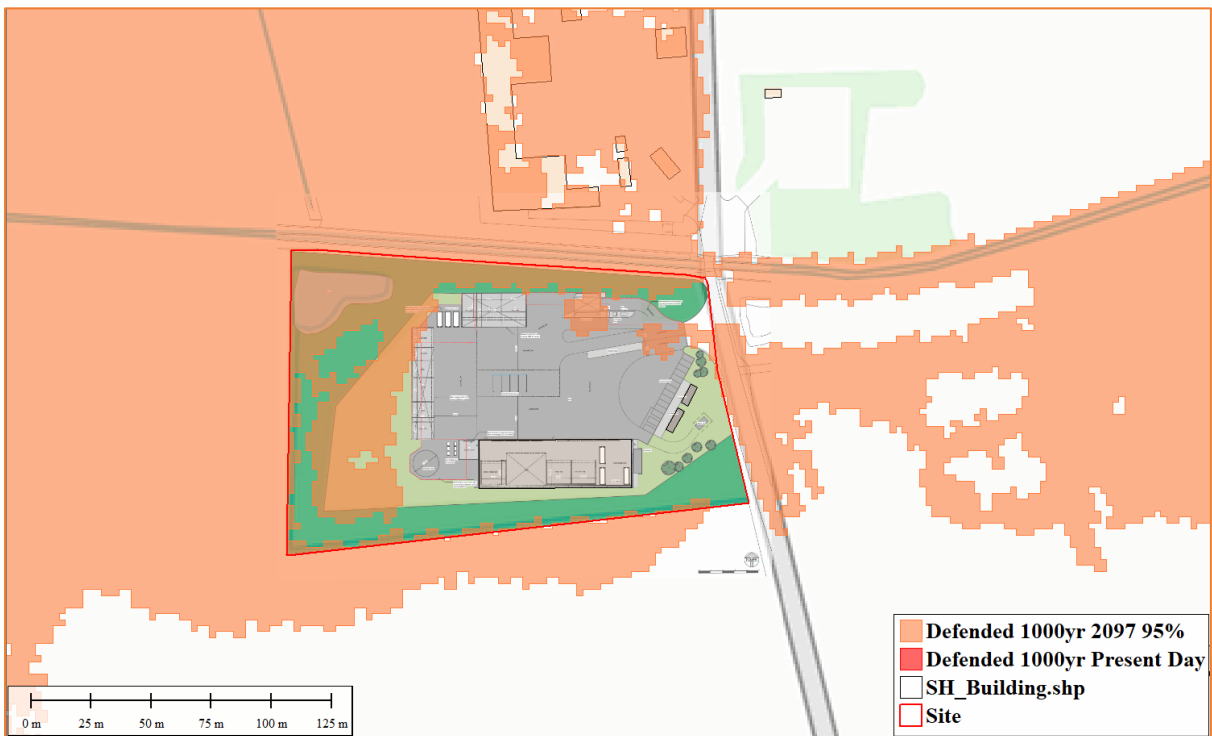
Figure 10: Modelled Point of Ayr to Pensarn defended 1:1000 year flood extents at the site (Source: NRW, OS Mapping, Proposed Site plan)
